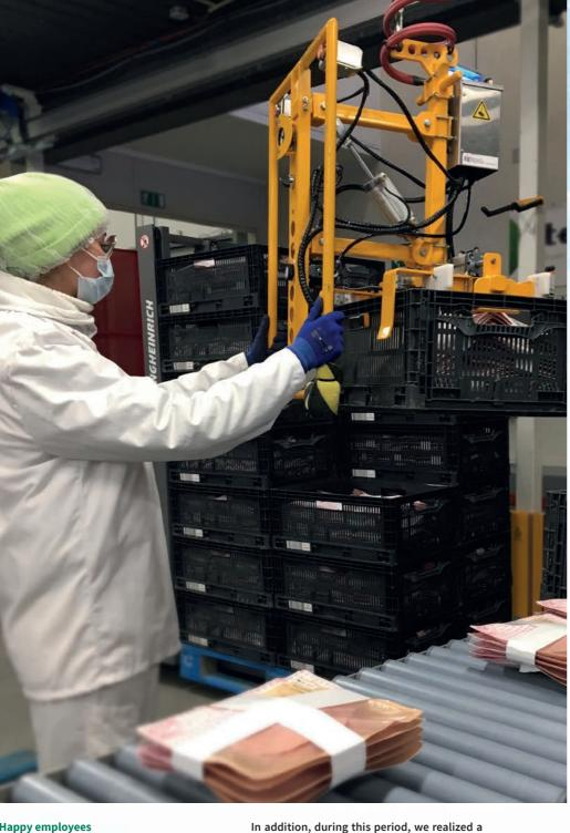
To improve the ergonomics and efficiency of our cutting lines, lifting equipment was installed on our lines. With this lifting solution, our employees are now able to lift 25 kg crates and stack them 8 high (instead of 6) on pallets.
